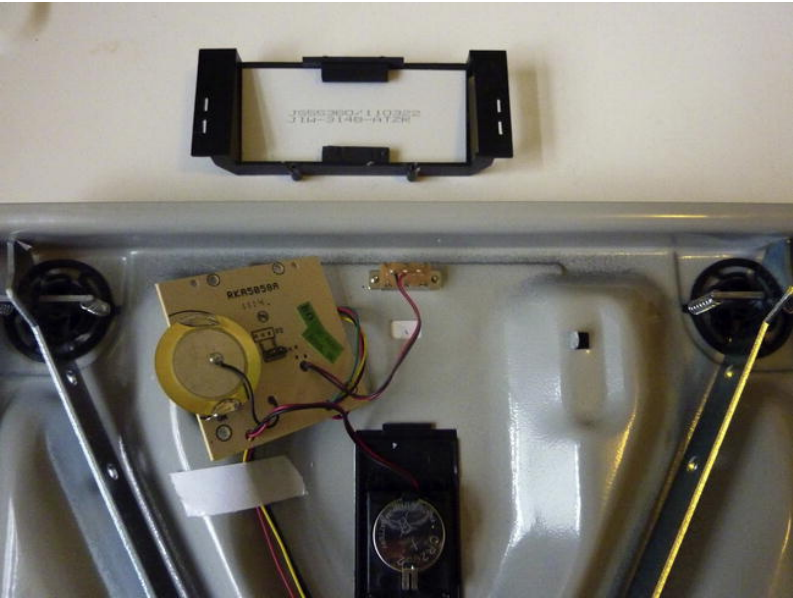
Figure 10-2. Scale after removing the cover and LCD
