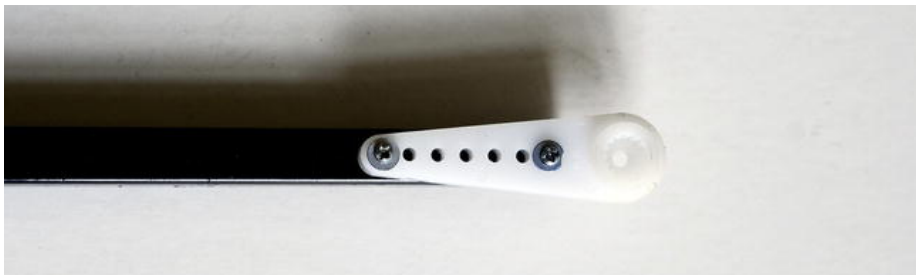
Figure 13-2. Thigh connected to the servo horn
