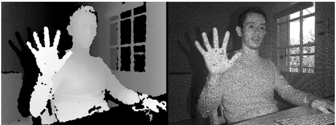
Figure 2-8. Depth map (left) reconstituted from the light coding infrared pattern (right)
