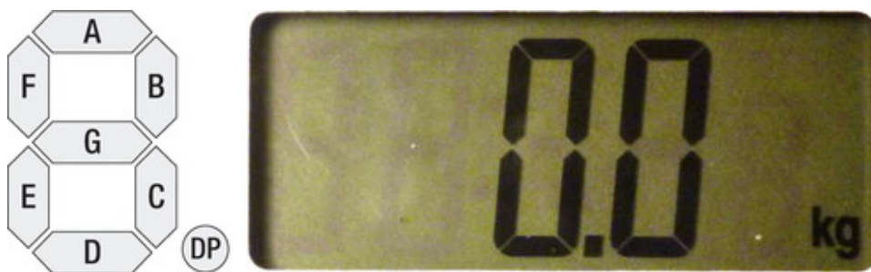
Figure 10-4. Individual segments (from Wikipedia), and the LCD on your scale.
