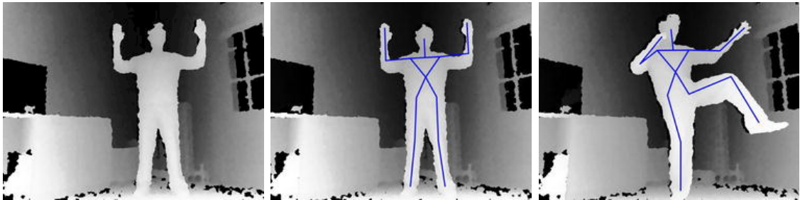
Figure 3-13. User in start pose, calibrated, and tracked
