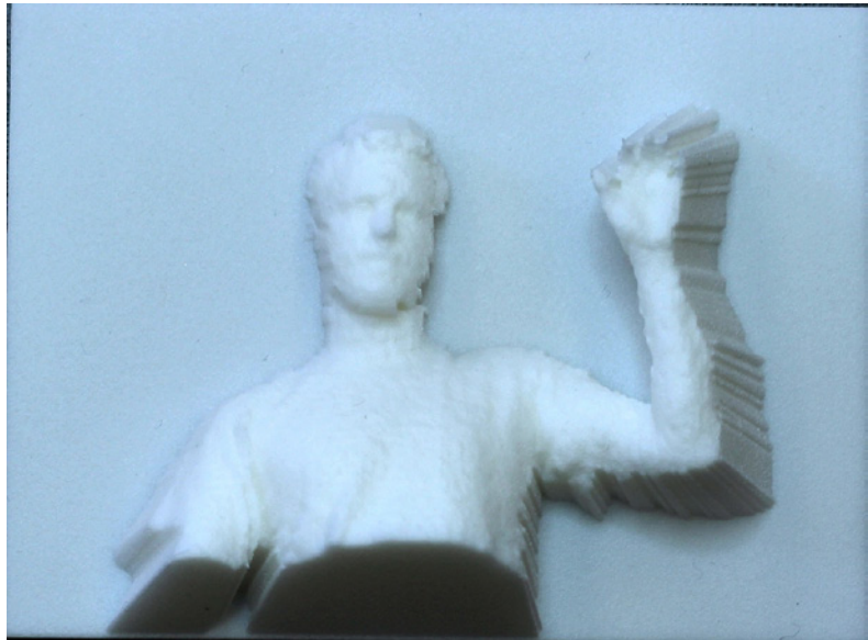
Figure 5-26. Final print received from Shapeways. Compared to the MakerBot print, the smooth surface of this print makes for much better results in the face and other areas of fine detail.
