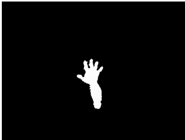
Figure 2-20. The depth image range is calibrated to capture only my hand.
