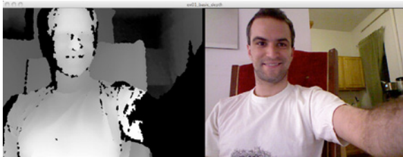
Figure 2-9. A screen capture of our first Processing sketch showing the depth image side by side with a color image from the Kinect.
