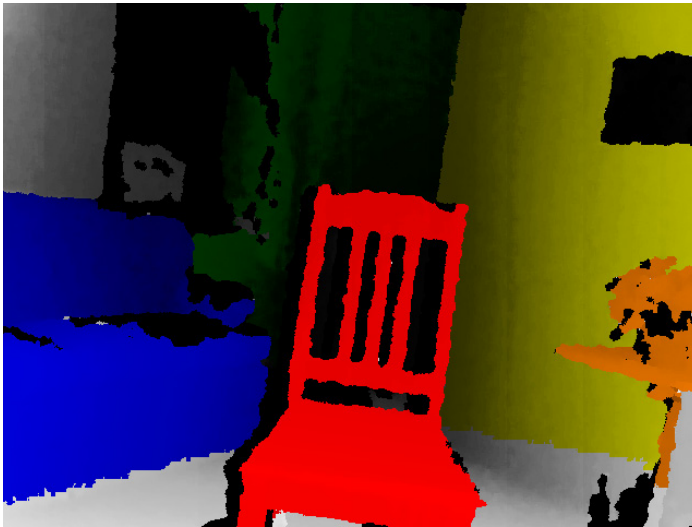
Figure 4-23. OpenNI's "scene map" breaks the depth map into spatially distinct pieces such as walls, people, and pieces of furniture. Here it is displayed mixed with the depth image to indicate separate objects.
