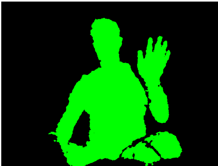
Figure 4-21. Separating the user pixels from the background pixels using getUsersPixels .
