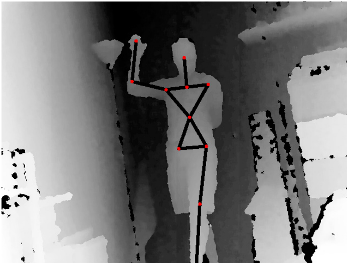
Figure 4-11. If the confidence score is too low for the given joints, SimpleOpenNI 's drawLimb function will hide the affected limbs—in this case, my left upper and lower arm and my right thigh and shin.
