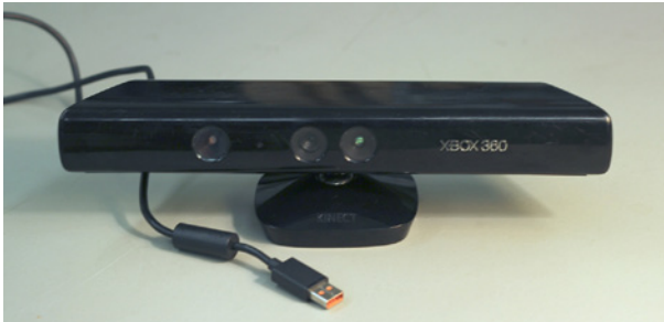
Figure 2-5. The Kinect has one wire coming off of it with a male Xbox connector at the end. This plugs into the female Xbox connector attached to the power plug.
