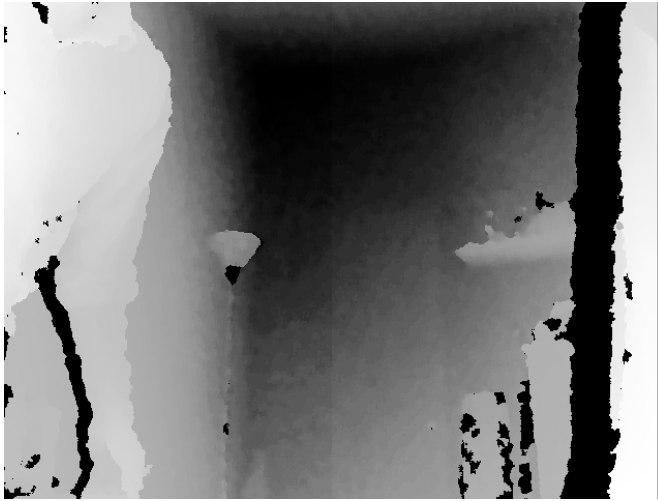
Figure 4-2. OpenNI can tell that a user is in the scene very early. This screen capture was taken from within the onNewUser callback, and you can see I've barely entered the frame on the left.
