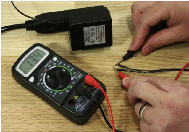
Figure 7-11. Measuring AC adapter voltage
