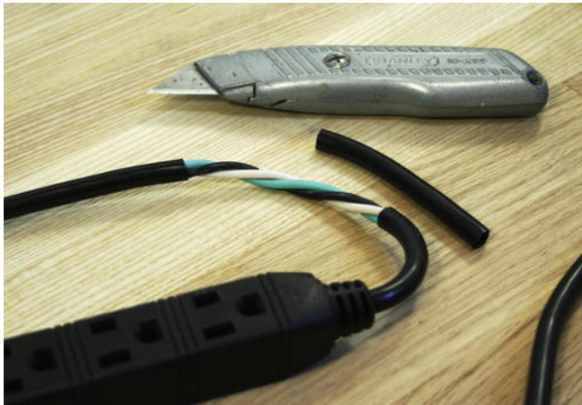
Figure 7-6. Outer insulation removed from power cable
