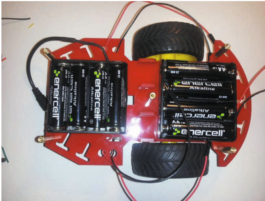
Figure 32-1. Add batteries to both of the battery holders (at this point no motors are connected)
