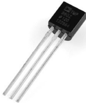
Figure 10-1. A temperature sensor is a tiny device; this is close to its actual size
