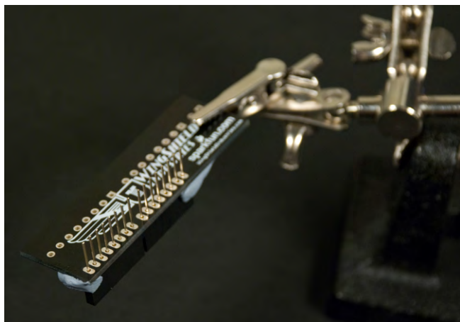
Figure A-3. Headers ready to be soldered
