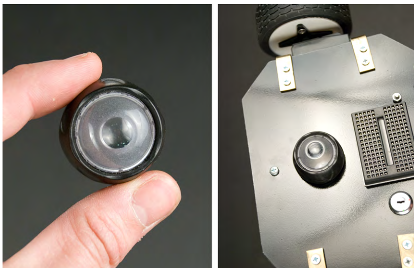
Figure 1-17. Lens glued on top of the chassis
