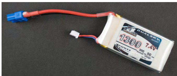
Figure 2-11. Rechargeable lithium-polymer battery pack
