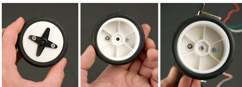
Figure 1-15. Servo horn attached to the tire rim and wheel attached to the servo
