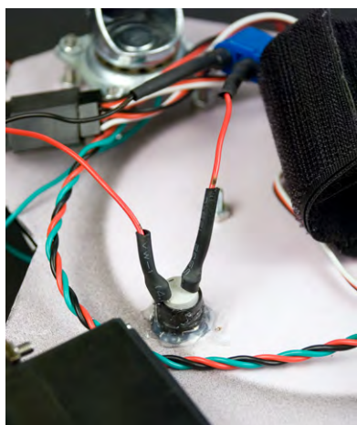
Figure 2-15. Positive wires soldered to the power switch
