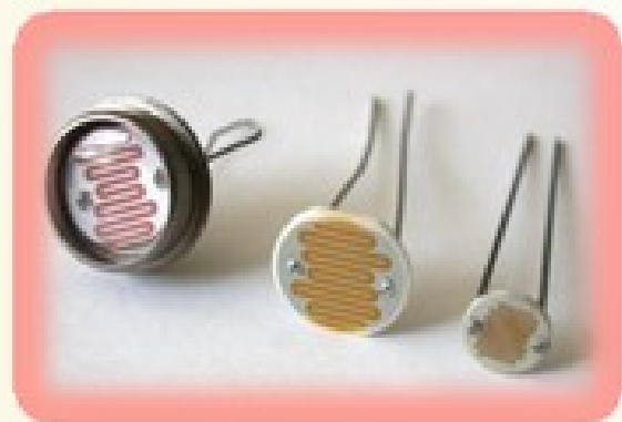
Photocell (light sensor)
