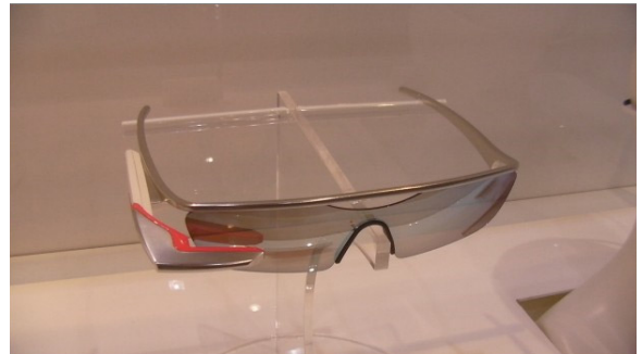
FIGURE 14-8: The NTT DoCoMo / Olympus lightweight mobile AR prototype (Photo courtesy of www.crunchgear.com )
