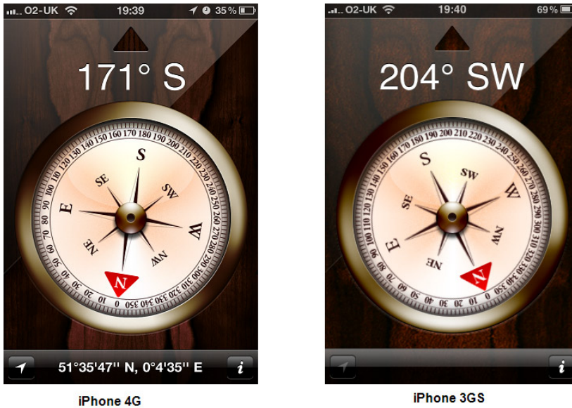
FIGURE 3-50: iPhone compass experiment with interference
